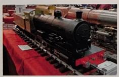
I have been in the hobby since the age of 8. I've entered IMLEC on a number of occasions, placing 1<sup>st</sup> in 2011 and best 3½" in 2010. This LNER Q5 was built over a 5 year period based on LBSCs "Netta", with many changes. Some of those are; balanced slide valves, helix exhaust with expansion chamber, increased radiant superheat, larger cylinders with larger passages and redesigned valve
