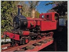
"Peveril" is a 5" gauge model of a class of Beyer Peacock 2-4-0 tank engines built for the Isle of Man Railway in 1875. The full sized engine is at the Railway Museum at Port Erin.
