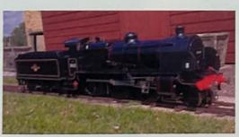
5" gauge Ex SR BR 'U' Class Mogul, based on Martin Evans "Ashford" design with modifications to represent a reasonably accurate "new build" U Class as opposed to a rebuilt "River" Class. Cast iron cylinders with rings on pistons and piston valves, 2 injectors for boiler feed.
