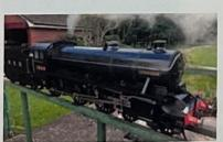
My loco was built in 1996 I have only owned it since last September I've had new piston valves fitted and new piston rings so hopefully all is good The loco is built to the Martin Evans design in black livery.
