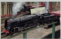
3½" gauge British Railways Standard Class 9F 92118 'Single Chimney' 2-10-0. Based on the design by LBSC and then Martin Evans. She was originally numbered and named as the '92220 Evening Star' with the 'Pines Express' name plaque, which has been changed due to the single chimney. A fantastic engine with an Ellis Professional Boiler, and
