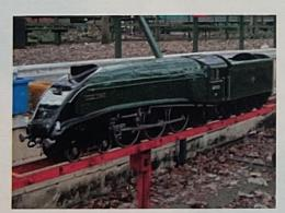
Built over a period of 4 years by the owner, roughly to Michael Breeze drawings. The only castings used were those for the 6 coupled wheels, everything else was either from solid or fabricated by the builder. The engine has run in 5 previous IMLECs, the best being 6<sup>th</sup> at Bournemouth and the worst half a lap at Leyland. It is quite a capable engine, the problem is with the driver!
