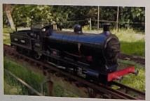
My Netta first showed it's smoke box at the 2003 Bristol IMLEC where it quickly blew a superheater. The firebox is full of radiant superheaters and brick arch. Fire tubes brought back an inch and now wish they were brought back a little further than on the plans. It's either coal hungry or the driver is addicted to shovelling.
