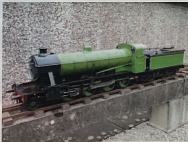
5" Gauge 2 – 8 – 0 O1 design Built & owned by Peter Wardle Completed 44 years, 2 boilers and 2000 miles ago, the loco is being driven by Birmingham SME member
