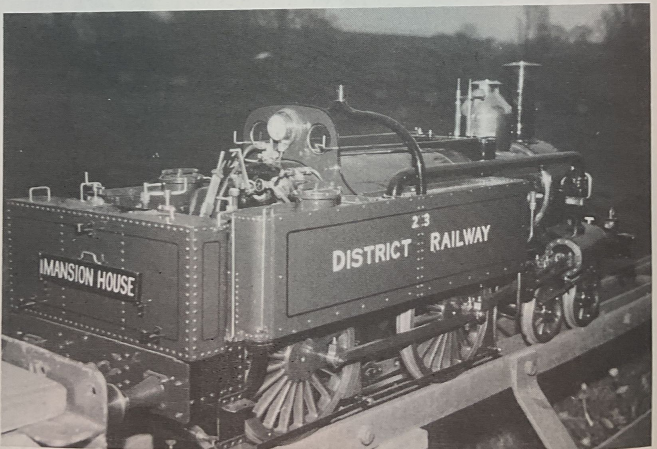
D. G. Sutcliffe's Beyer-Peacock District Tank. These engines were fitted with condensers to allow working underground
